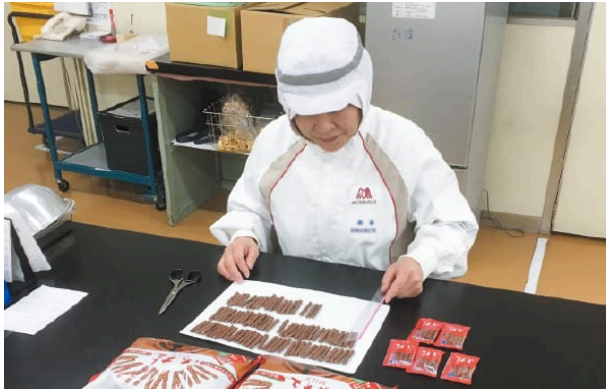
Shipping inspection (measuring that dimensions and weight meet product standards)
